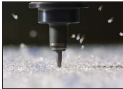
The standard 10,000-rpm spindle is perfect for routing aluminum, plastic and other light materials. An optional 15,000-rpm or high-torque 5000-rpm spindle are also available.
