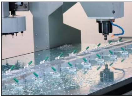
A powerful 40-taper milling head, 10-pocket tool changer and large travels make quick work of long extrusions and large sheets of material.
